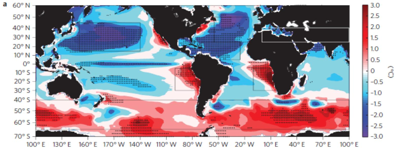
Wang et al. 2014 | **Annual-mean SST bias averaged in 22 climate models.** The SST bias is calculated by the SST difference between the model SST and extended reconstructed SST.
