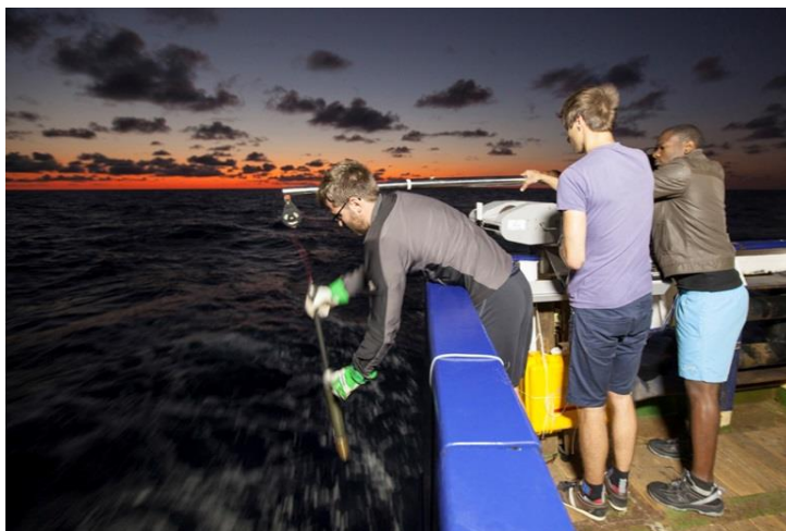
Fig. 1: Underway-CTD measurements on FS METEOR. Robert Kopte is recovering the probe after collecting a CTD profile. Amaro Francisco and Jonas Boomers are assisting by keeping the gibbet of the winch in the right position. (Photo: Thilo Klenz)
